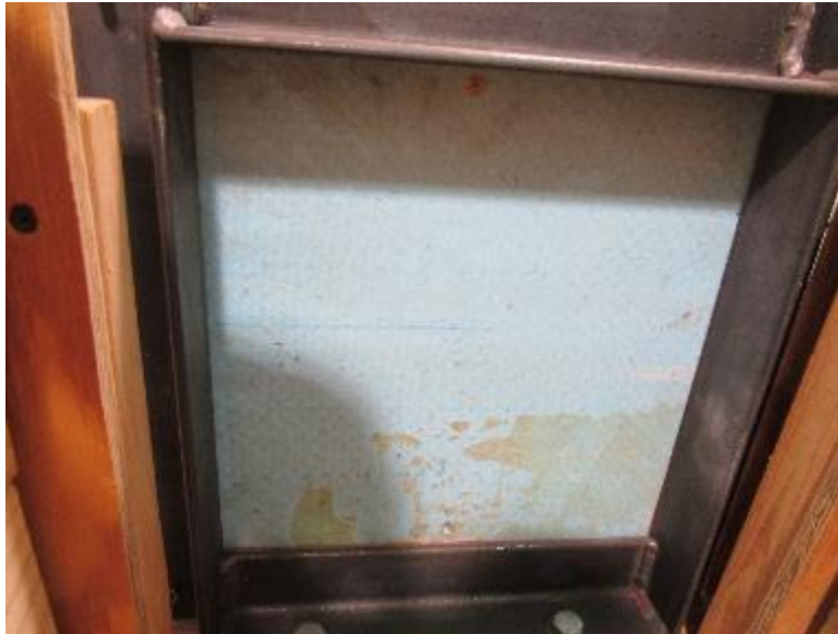
Photo No. 2 UL 752, Level 8, Pre-Test Interior
